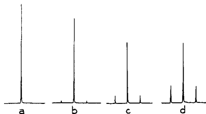
Figure 1. Aldehyde proton resonance (400 MHz) for \text{RhCl}(\text{CO})(\text{PPh}_3)_2 + {}^{13}\text{CO} + \text{PhCHO} in \text{C}_6\text{D}_6 showing successive incorporation of {}^{13}\text{C} isotope into benzaldehyde. The resonance is at \delta 9.63 ppm with J(^{13}\text{C}-\text{H}) of 173 Hz. Irradiation times: (a) t = 0 ; (b) 1 day; (c) 5 days; (d) 10 days.
